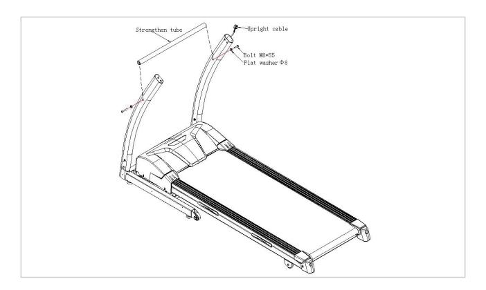
• Fix the strengthen tube to the uprights with bolts and washers.
