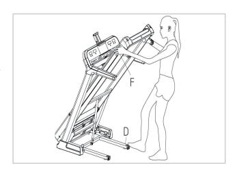
To tilt, start by placing one hand at position "F" to support the top end of the treadmill. Next, place one foot at position "D" to hold the bottom end of the treadmill steady. With your foot at "D", slowly tilt the top of the treadmill downward towards the ground. Once the Main Frame "F" reaches a low enough point, the wheels of the treadmill will become active.
