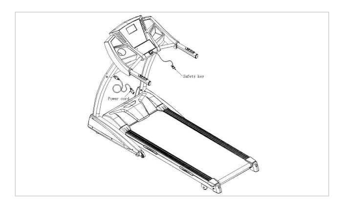
• Put on the power cord and safety key, then power on the machine.
