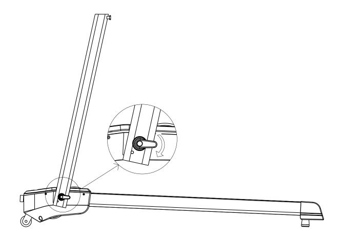
After finishing the uplifting, screw the hand knob according to the direction as the arrow shows.
