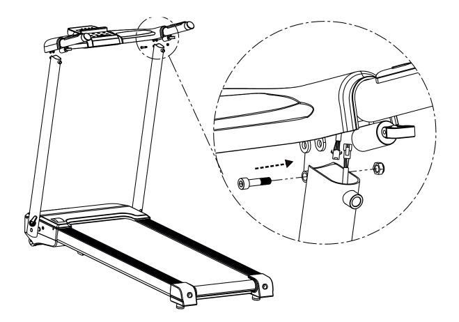
Use the M6 screws (the screw is pre-assembled on the upright tubes) to fix the console together with the upright tubes, then connect the connector wires of the right handrail and upright tube.
