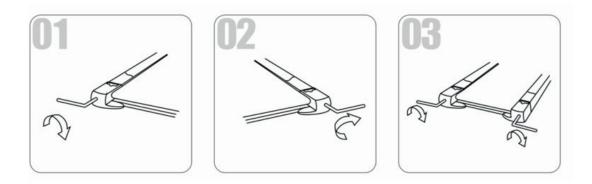
(1) Running belt deviates to left - Start the machine, set speed at 2-3 km/h without a load on the belt, use Allen key to turn the screw 1/4 turn (see fig. 1). Then allow the machine to run without a load for 1-2 minutes. Repeat process until the belt becomes central.
