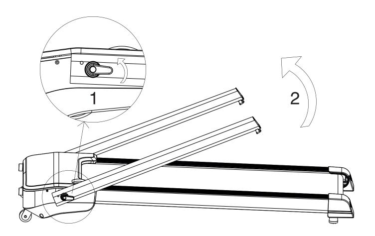
1. Unscrew the adjusting knob on the both sides of the frame respectively (suggest unscrew 3 circles) to make lower ends of upright tubes flick from the main frame.
