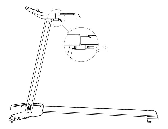
Put the handrails of the console in the horizontal direction and clip the pull pin of the left and right handrails into the holes on the upright tubes.
