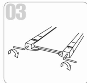
**01. Running belt deviates to left:** Start the machine, set speed at 2-3 km/h without a load on the belt, use Allen key to turn the screw 1/4 turn (see fig. 1). Then allow the machine to run without a load for 1-2 minutes. Repeat process until the belt becomes central.
