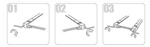
**01. Running belt deviates to left:** Start the machine, set speed at 2-3 km/h without a load on the belt, use Allen key to turn the screw 1/4 turn (see fig. 1). Then allow the machine to run without a load for 1-2 minutes. Repeat process until the belt becomes central.
