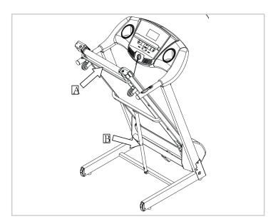
Hold the position A, pull up the machine, till cylinder gets the position B.
